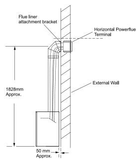
**Horizontally Terminated:** Utilises the escea horizontal power flue enclosure kit.
