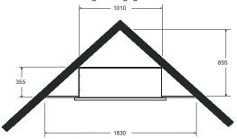
NOTE: Allowances need to be made for cladding the internal of the cavity.
