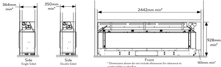
Note: These are minimum cavity framing dimensions and may not achieve a centred fireplace design in all specifications. Please adjust overall cavity size if required.
