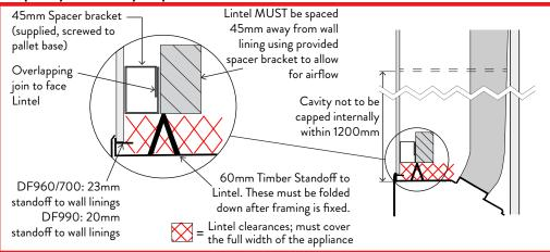
\*WARNING: The top standoffs must be adjusted to the upright position before the fireplace installation. All standoffs must remain in place for fireplace installation and then folded down once framing is fixed.
