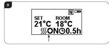
Note: It is normal for the fan heater to stop running for periods of time. This happens if the room temperature is higher than the temperature set on the control.
