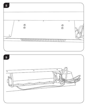
8.7 Replace in reverse order ensuring the wires are put back in exactly the same configuration.
