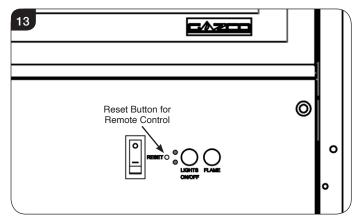
Resetting of the remote control is necessary if the appliance operates wrongly due to external interference signal and the remote control is not in use.
