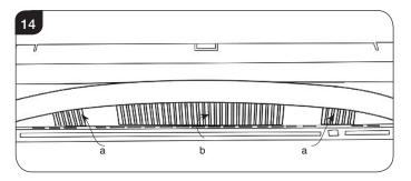
Dust build-up can inhibit efficient performance of the fan and lead to the safety cut-out operating.
